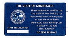
Example prefab construction label - located under kitchen sink.
